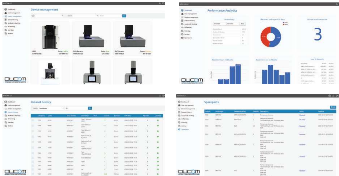
Figure 4. Few features available on the MOOHA web-based software: performance analytics, device management, dataset history (digital log book), spare parts and a lot more.
