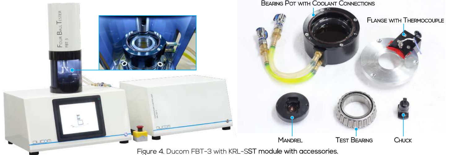
Figure 4. Ducom FBT-3 with KRL-SST module with accessories.
