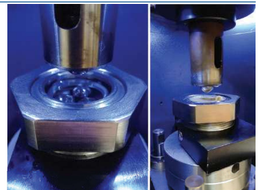
Ball pot ready for test in oil (left) and grease (right).
